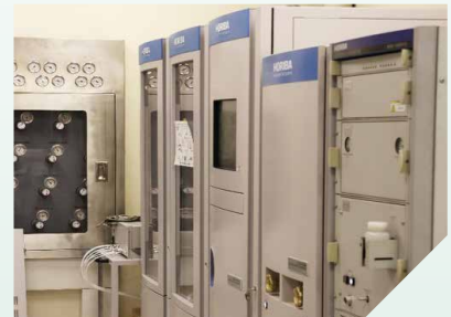
Various measurement and analytical instruments used to determine a vehicle's emissions and other pollutants that can adversely affect the environment.
